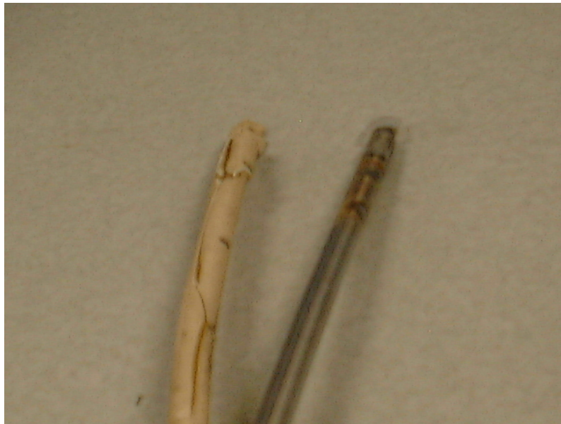
Figure 6: Photograph of failed thermocouple and PVC sheath.
